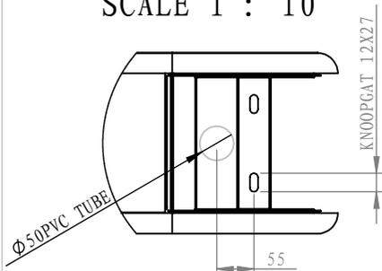
**EXPANSION BOLT IS INSTALLED IN ELLIPSE TO FIX THE EQUIPMENT, AND CONTROL LINE AND POWER LINE ARE IMPORTED FROM Ø50PVC**
